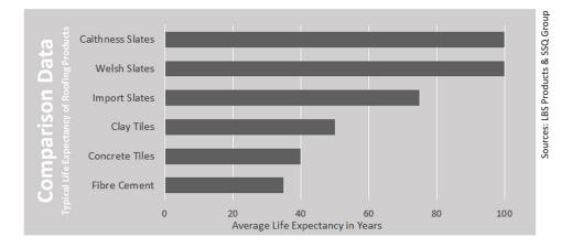
Outperforming almost all other alternative roofing materials in terms of durablity, Caithness flagstone roofing is made to last.
